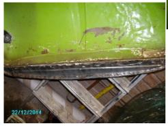
indent using 2 sockets one smaller than the other and a big hammer!.
